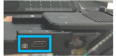
The shutter release for Sony Cameras is Type-C to Multit, and the shutter release cable for Panasonic is Type-C to DC2.5mm. (For more details, please refer to the compatibility list)
